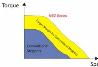
Due to closed loop control and adoption of advanced control algorithm, the MEZ series servo systems can always implement 100% torque of the motor, and do not need the huge 50% torque reservation in normal open-loop stepper systems. This feature significantly improves system high speed performance. While open-loop stepper systems are typically adopted in applications under 1,000 rpm, the MEZ series servo systems are ideal for many applications up to 2,000 RPM, sometimes even to 3,000 RPM!
