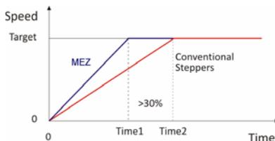
Also due to closed loop control and adoption of advanced control algorithm, the MEZ series servo systems can always implement 100% torque of the motor. This feature significantly improves system response or acceleration performance, usually up to 30% quicker or higher acceleration than a same size and holding torque conventional steppers.
