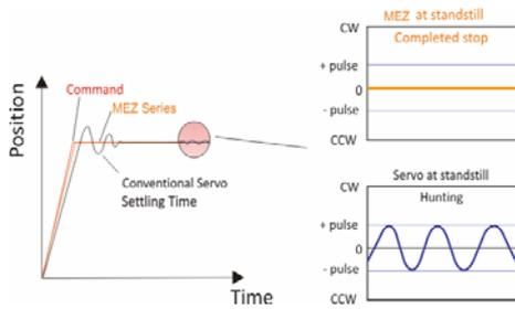
For the case of conventional servo motor systems, there is a considerable delay between the commanding input signals and the resultant motion because of the constant monitor of the current position, necessitating a waiting time until it settles, called settle time.
